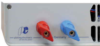
DC oval flat clamp in front panel
